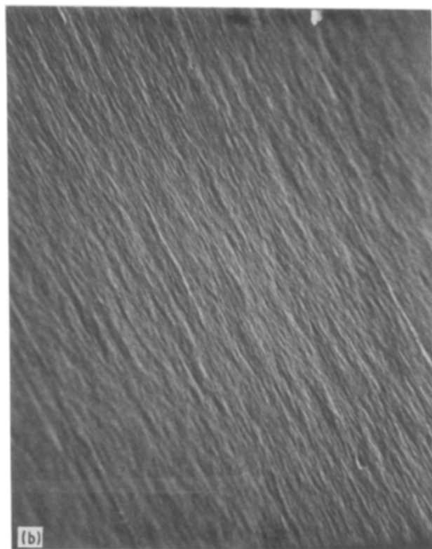
Figure 9 SEM micrographs (× 5000) showing fracture surfaces of (a) neat epoxy; and intercrosslinked epoxy-bismaleimide networks (b) 25:75, (c) 50:50, (d) 75:25.
